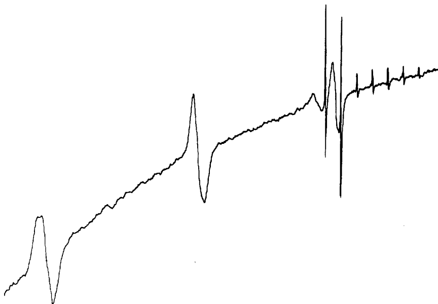
Figure 2. Recorded trace of the differential of the nuclear resonance lines in \text{PrVO}_4 at 4.2 K and a frequency of 12.916 MHz. The external field is applied along the [001] axis. The broad lines are from ^{141}\text{Pr} ( I = \frac{5}{2} ), the narrow lines from ^{51}\text{V} ( I = \frac{5}{2} ). The latter are saturated except where they are sufficiently close to a praseodymium line for cross-relaxation to occur.
